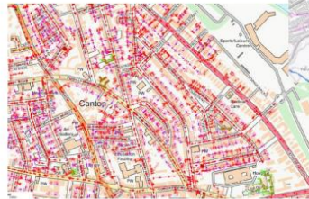
Pontcanna combined network. Note no outfalls to the River Taff.
