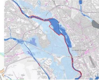
Pontcanna combined network. Note no outfalls to the River Taff.
