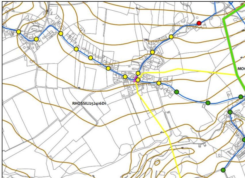
Figure 3 - Example conceptual output from Project Nemo, coloured symbols represent likely location of a leak
