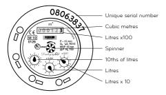
Spinner: Revolves fast when water is being used but may move slowly if you have a small leak, a dripping tap, or if a ball valve is in the process of closing.
