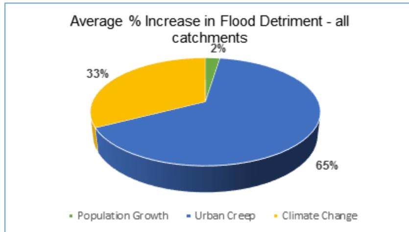
**Figure 4: Results of hydraulic modelling analysis (average % increase in flood detriment for all catchments – rationalised)**
