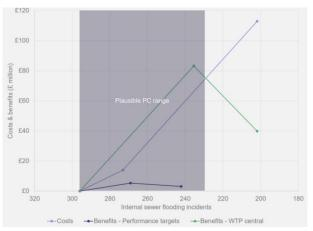
Figure 3 Internal sewer flooding - cost curve from cost benefit analysis
