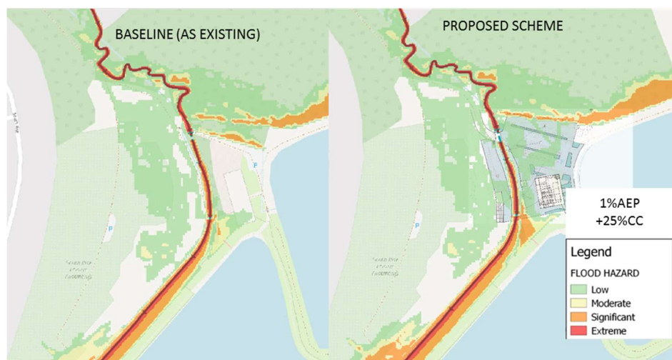
Figure 4-3 – Comparison of baseline and proposed scheme flood extents (1% AEP +25% climate change event)
