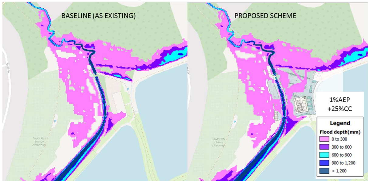
Figure 4-2 – Comparison of baseline and proposed scheme flood extents (1% AEP +25% climate change event)
